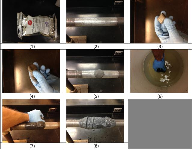
Figure 1. Example of Stop It Repair
