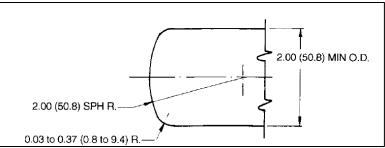
Figure 4. Tup Nose Detail
