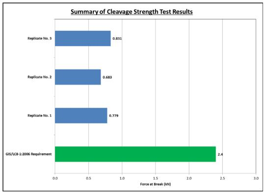
Figure 2. Summary of Cleavage Strength Test Results (Product #3)
