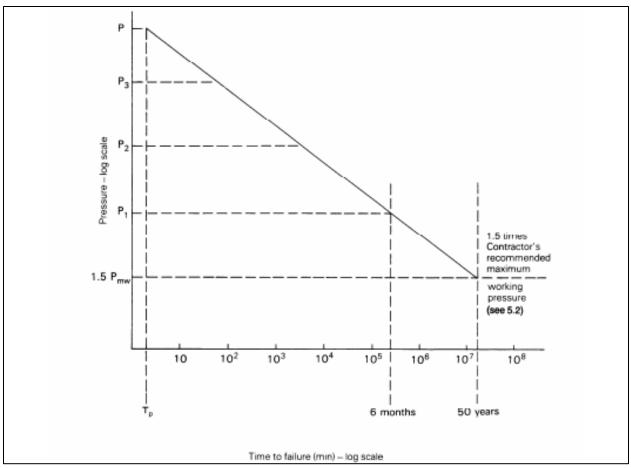
**Figure 6. Pressure/Life Testing<sup>3</sup>**
