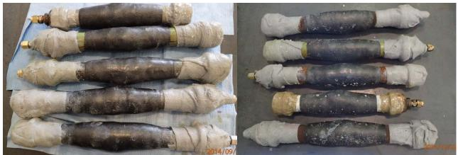
Figure 5. Repaired Specimens with IPI Stop It before (left) and after (right) Cyclic Corrosion Test
