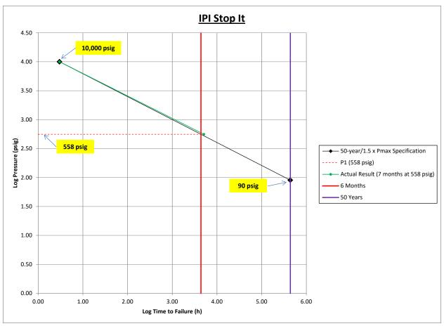
Figure 8. Long-Term Pressure Test Results for Stop It Repaired Specimens
