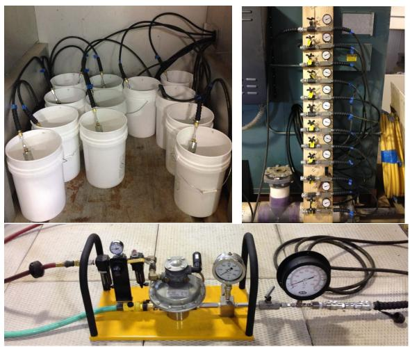
Figure 7. Long-Term Pressure Testing Setup
