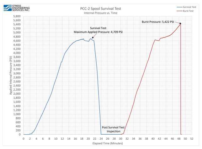
Figure 4: Plot of internal pressure vs elapsed time for survival and burst test
