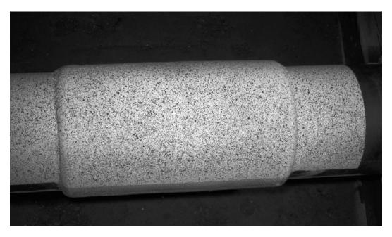
Figure 3: Pipe spool survival specimen with stochastic speckle pattern applied for DIC imaging
