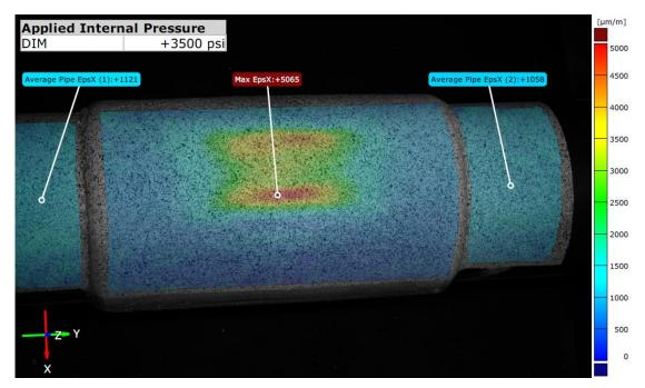
Figure 6: Overlay of composite repair and pipe body hoop strain at 3,500 PSI acquired using DIC during pipe spool survival pressure test.
