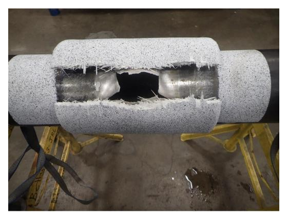
Figure 5: Photograph of sample following spool survival and burst test, isllustrating failure in machined wall loss region
