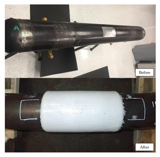
Figure 2: Photograph of pipe spool survival specimen before and after repair installation
