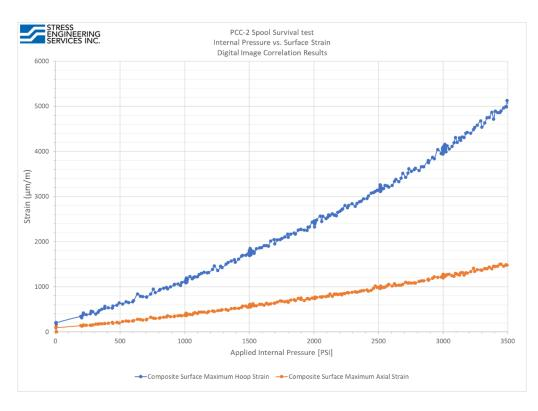
Figure 9: Plot of recorded composite repair strains acquired using DIC vs. internal pressure
